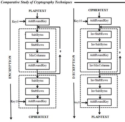
Figure 2: AES Encryption and Decryption
