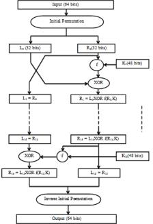
Figure 1: Diagram of DES Algorithm
