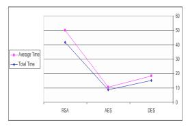
Figure 2 Total and average time for encryption
