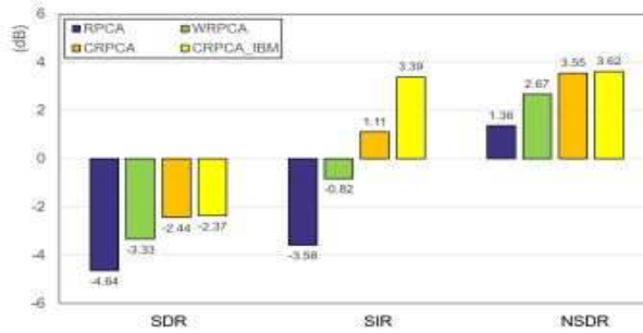
Figure 2. A comparison of RPCA, WRPCA, CRPCA, and CRPCA on SDR, SIR, and NSDR on our dataset with IBM.
